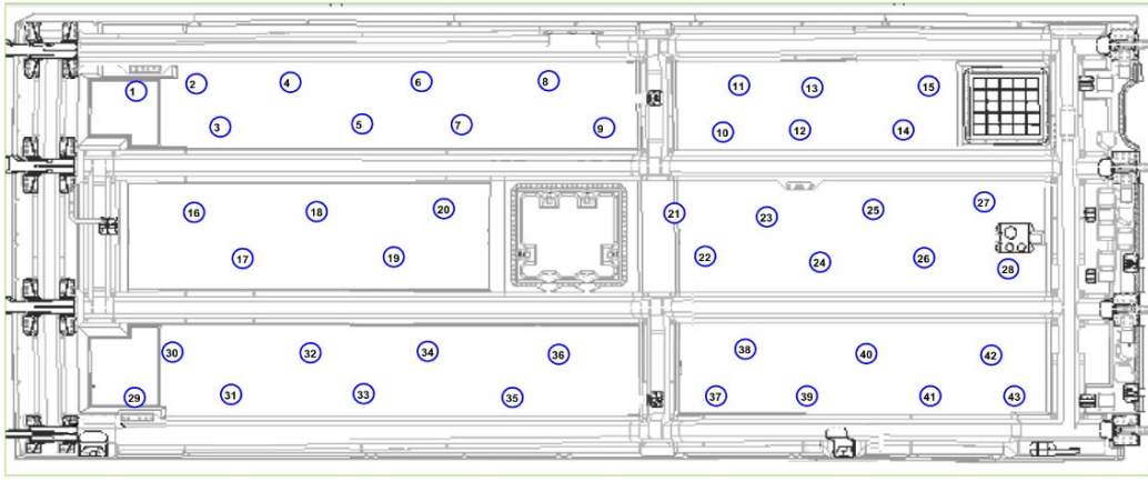
Figure 3: PZT deployments on the Fan Cowl Structure on an instrumented A380.
