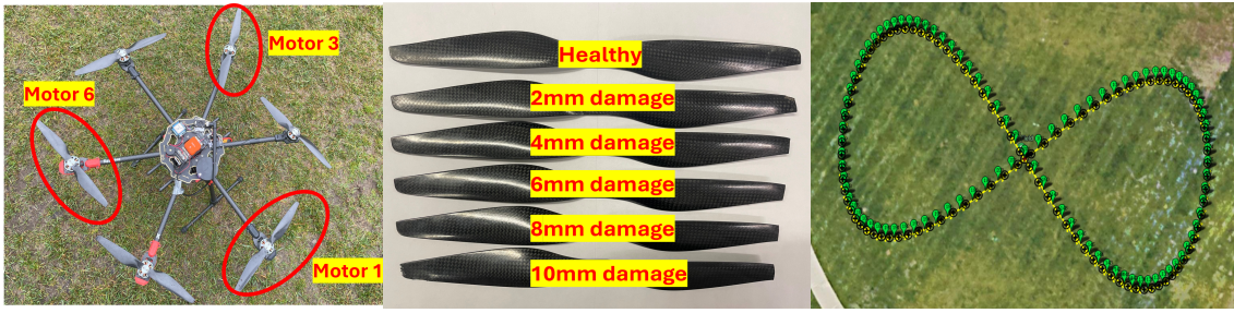
Figure 1. (Left) The Hexacopter used for data collection. (Middle) Healthy and damaged propellers with tips clipped off by 2 ~ 10 mm with 2 mm increment. (Right) Waypoints are designed to approximate an 8-pattern flight path.
