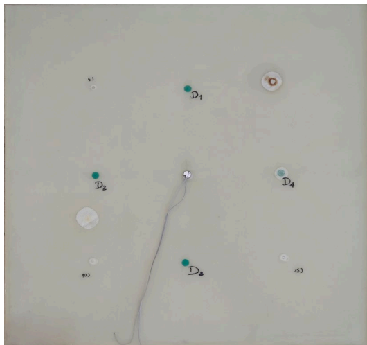
Figure 2. Experimental specimen: the GFRP laminated plate with multiple delaminations
