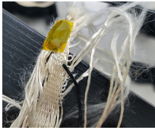
Figure 7B. Close-up of frayed and broken Vectran fibers around sensor package after pulling to failure.
