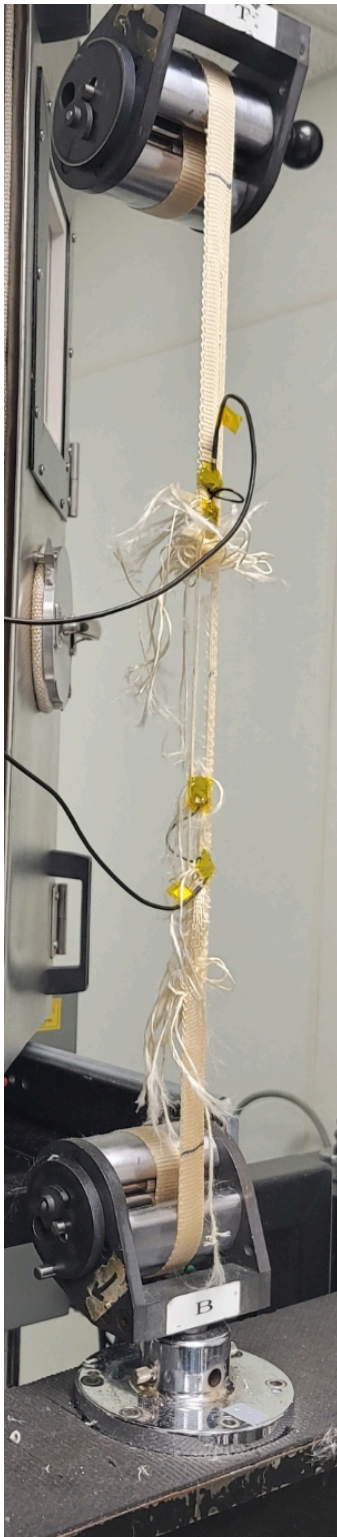
Figure 7A. Broken Vectran strip after pulling to failure.
