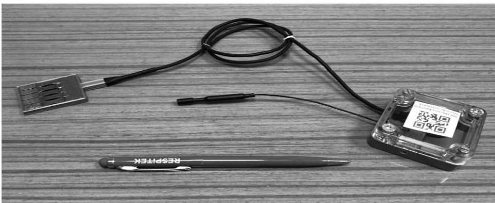
Figure 1. A general view of the Active(With Battery) Fatigue Sensor (US 8,746,077 B2) [12]
