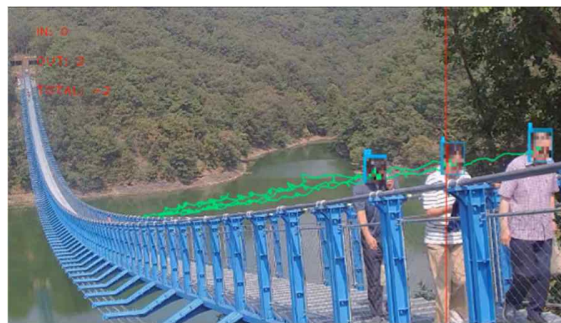
Figure 2. Pedestrian counting scheme using YOLO and SORT.
