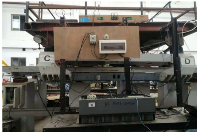
Figure 5. Mixed Suspension Control System Test Stand
