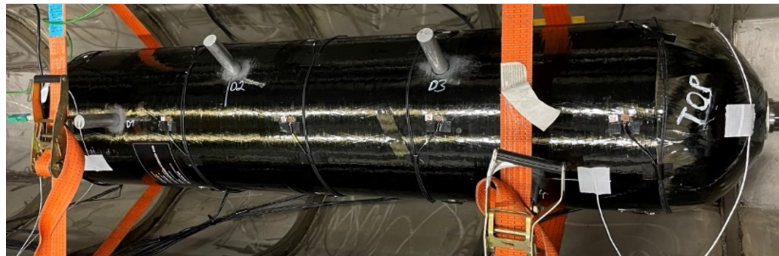
Figure 1. Overview of the sensor placement and reversible damage positions (D1-D4) on the unwrapped COPV without dome areas. COPV with four masses glued onto the surface as artificial damage on different positions (D1-D4)
