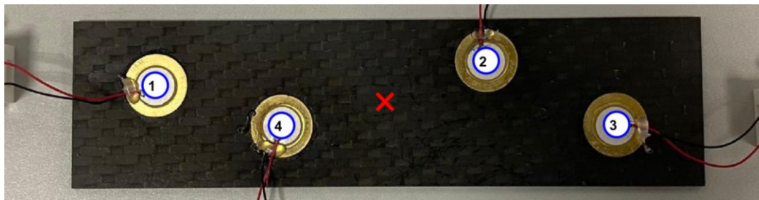
Figure 3: Composite coupon sample equipped with four PZT transducers. The red cross denotes the position at which the laser shock has been achieved.
