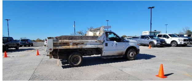
Figure 2. The truck on the slab in a static load test.
