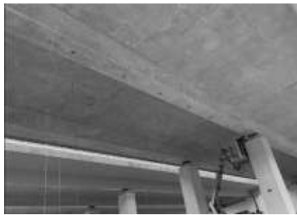
Figure 4. 24-channel AE measurement system with cabling and VS-30 sensors installed on selected elements of the viaduct.
