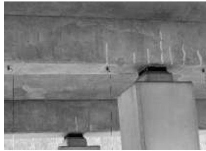
Figure 4. 24-channel AE measurement system with cabling and VS-30 sensors installed on selected elements of the viaduct.
