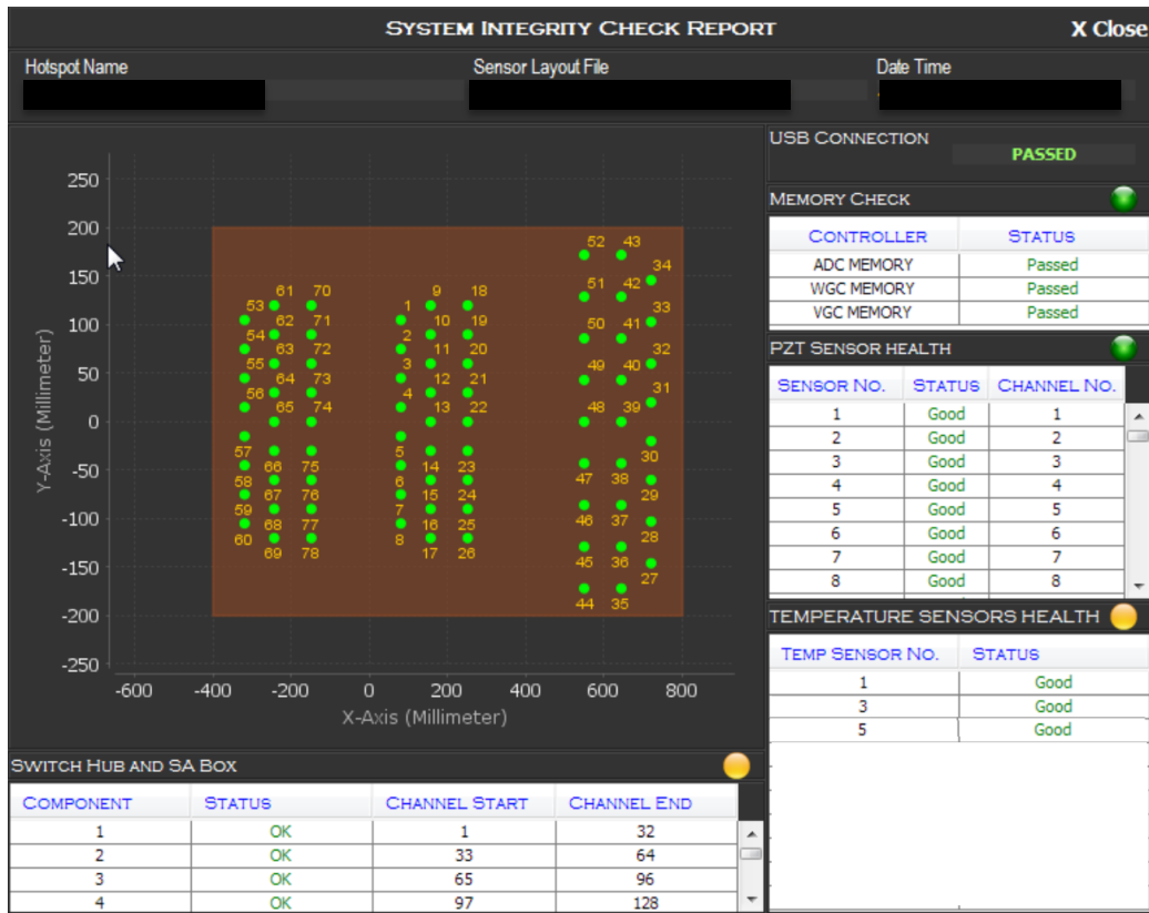
Figure 6. System integrity check after sensor installation and cable connections
